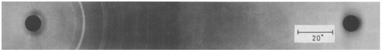
Figure 1 X-ray powder photograph of bulk  $\text{Se}_{20}\text{Te}_{80}$  alloy.
